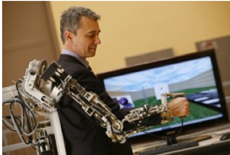
Figure 2.4: Photo of the exoskeleton ABLE worn by P. Garrec (credit to CEA-LIST) (Garrec, 2010)
