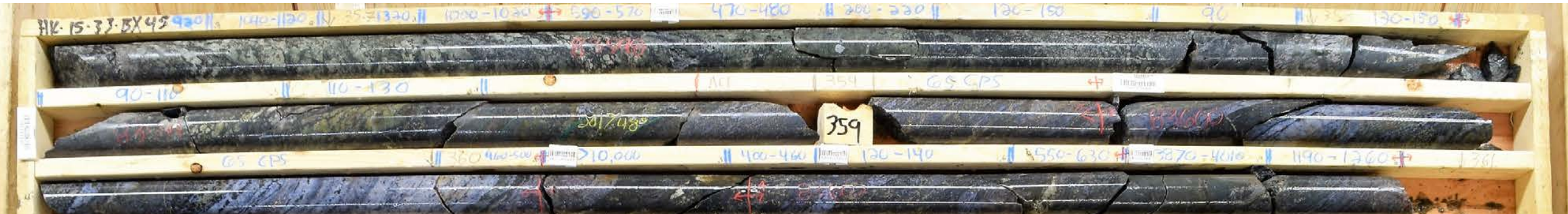
Isolated veinlets with dark infill (chlorite)
