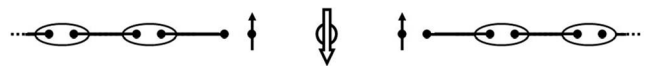
FIG. 13. Spin-1 chain with a Cu spin- \frac{1}{2} defect. Spin- \frac{1}{2} states are formed on either side of the Cu atom and align to form a spin-1 state.
