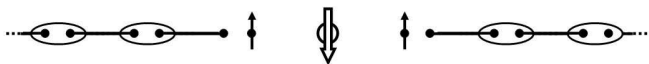
FIG. 13 Spin-1 chain with a Cu spin-1/2 defect. Spin-1/2 states are formed on either side of the Cu atom and align to form a spin-1 state.
