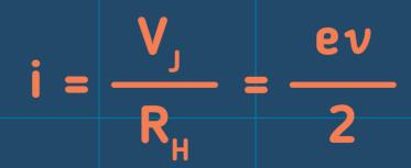
Force the elementary electrical charge of an electron  $e = 1.602 \ 176 \ 634 \ 10^{-19} \ C$  and measure the frequency ( $\nu$ ): you have now a way to measure a current in ampere.
