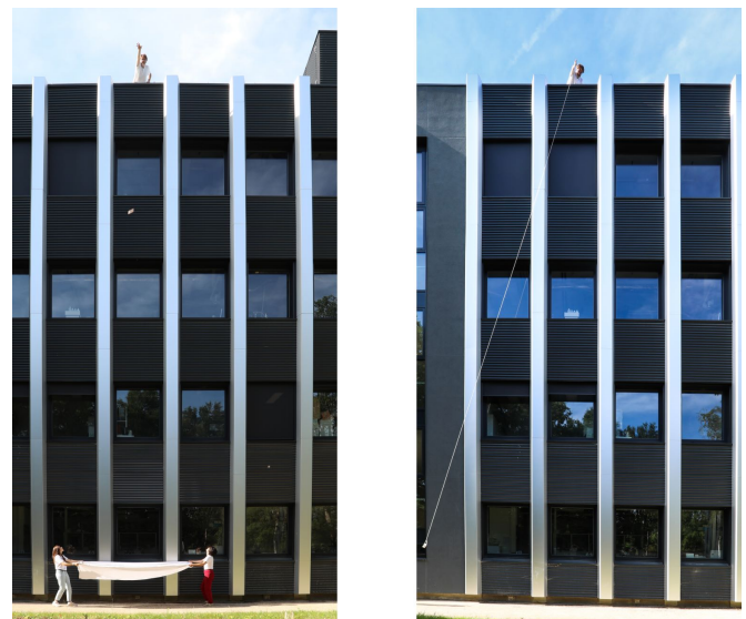
Figure 1: Measurement of the height of the building using method #1 (free fall of a smartphone) and #13 (giant pendulum, using the smartphone's gyroscope). Results are presented in Table 1.
