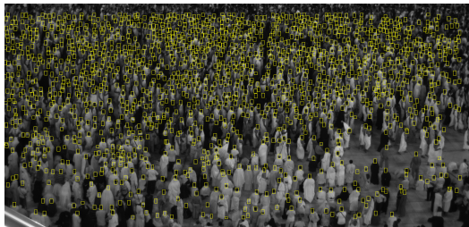
Fig. 2: Example of detection results of the RetinaNet, with ResNet-50 as architecture. Multiple factors such as the density, occlusion level and homogeneity of the scene impede significantly the tracking process.
