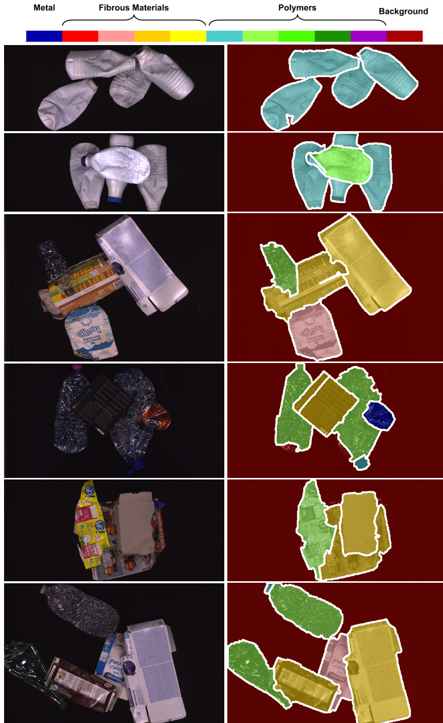
Figure 3: First set of results: each line corresponds to a different scene, with RGB image (left column) and labeled object-segmentation result with colored labels overlaid on the gray-level intensity image (right column).
