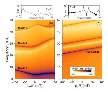
FIG. 3. (Color online) Map of the power spectral density (PSD) of excitations as function of the applied static field  $H_z$  for  $D = 3 \text{ mJ/m}^2$ . (a) Single isolated skyrmion in ground state. (b) Nominally uniform ground state. FMR denotes the ferromagnetic resonance or uniform precession mode. The insets at the top show the corresponding PSD in zero static field,  $H_z = 0$ .
