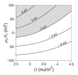
FIG. 1. Energy contours of  $\Delta U$  related to the metastability of the isolated skyrmion state with respect to the quasiuniform state.  $\Delta U > 0$  indicates a lower energy for the quasiuniform state, while  $\Delta U < 0$  indicates a lower energy for the isolated skyrmion state.
