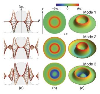
FIG. 4. (Color online) Spatial profiles the fluctuation in the magnetization component  $\delta m_z$  of the skyrmion breathing modes for  $D = 3 \text{ mJ/m}^2$  at  $\mu_0 H_z = 0 \text{ mT}$ . (a) Spatial profile of the fluctuation across the dot, where each curve represents a different instant *t* over one period of oscillation with the static core profile given in grey. (b) A two-dimensional snapshot of the mode. (c) A three-dimensional snapshot of the mode.
