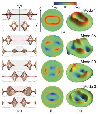
FIG. 6. (Color online) Spatial profiles of the skyrmion breathing modes for  $D = 4.5 \text{ mJ/m}^2$  at  $\mu_0 H_z = -75 \text{ mT.}$  (a) Spatial profile of the fluctuation across the dot, where each curve represents a different instant *t* over one period of oscillation with the static core profile given in grey. (b) A two-dimensional snapshot of the mode. (c) A three-dimensional snapshot of the mode.
