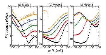
FIG. 5. (Color online) Mode frequency as a function of perpendicular applied field  $\mu_0 H_z$  for different strengths of the DMI, *D*. (a) Mode 1. (b) Mode 2, with a frequency splitting seen for  $D = 4.5 \text{ mJ/m}^2$  in the field region  $\mu_0 H_z \leq -60 \text{ mT.}$  (c) Mode 3.
