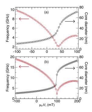
FIG. 7. (Color online) Variation of the breathing mode frequency (squares) and skyrmion core diameter (circles) as a function of the perpendicular applied static field  $\mu_0 H_z$ . (a) Micromagnetic parameters from Thiaville *et al.* [25]. (b) Micromagnetic parameters from Sampaio *et al.* [33].
