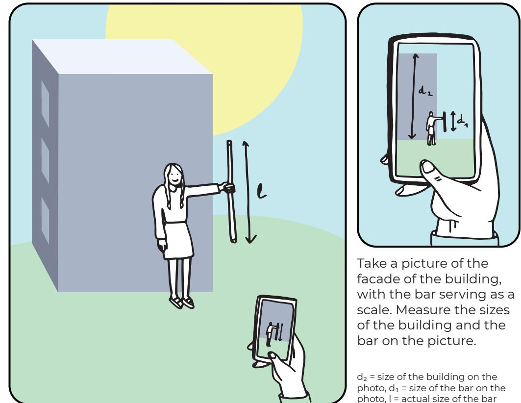
Take a picture of the facade of the building, with the bar serving as a scale. Measure the sizes of the building and the bar on the picture.
