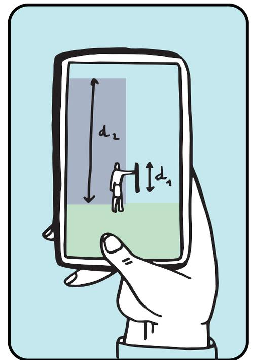
Take a picture of the facade of the building, with the bar serving as a scale. Measure the sizes of the building and the bar on the picture.
