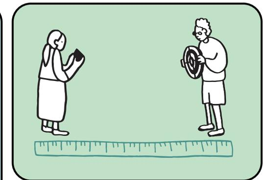
Install the target at the bottom of the building, and take a picture from the top of the building. The number of pixels representing the target in the picture varies in  $1/R^2$ , and must be calibrated before.
