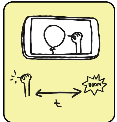
From the top of the building, film in "slow motion" the bursting of a balloon at the bottom of the building. Measure the time elapsed between the image and the sound of the exploding balloon.
