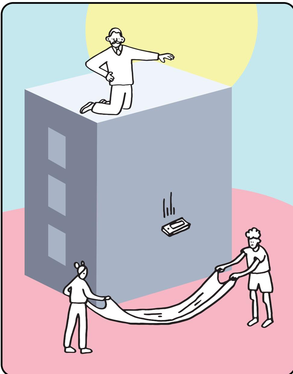
Drop your smartphone from the top of the building, your friends receiving it down in a sheet, like firefighters. The recording of the accelerometer data makes it possible to determine the time of fall, and if needed the value of the acceleration can be used to take air drag into account.
